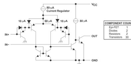
*The comparator compares two voltages, and if the + input one is higher than the other the output transistor is turned on, if not then off.*
