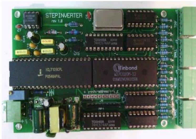
bits in rom. Low order ten bits of rom are continuously clocked from a 3.2768Mhz crystal oscillator module. The A/D converter starts a conversion every 40mS and its output is latched into the rom every second cycle right at the zero crossing.
