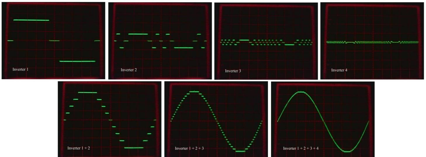
*A three inverter stepped system with 27 steps produces about 4% harmonic distortion, about the same as measured off the the grid here. A four inverter stepped system with 81 steps peak to peak produces just slightly below 1% measured harmonic distortion without any filtering.”*
