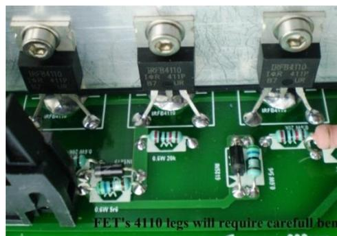
*Switching losses are added to the IR losses, ( and in anything I build usually outweigh the resistive losses hands down). Getting the switching losses down is a science unto itself... black science almost, add in parasitic oscillations and lots of other gremlins, and we have our work cut out to keep the losses less than the 370 watts. If we fail, it goes up in smoke.*
