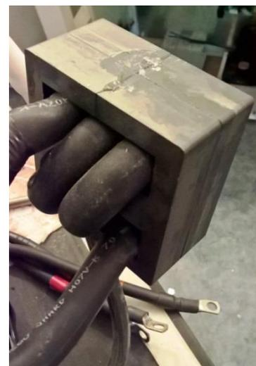
Voltage feedback may lose control. But if you get the transformer tuning exactly right (ideally +/- 1Hz) after fitting a really nice large non saturating steel cored choke into the primary, a great many problems will have been solved, and you will then have a sweet running and efficient inverter with a good clean low distortion sine wave at the output”.
