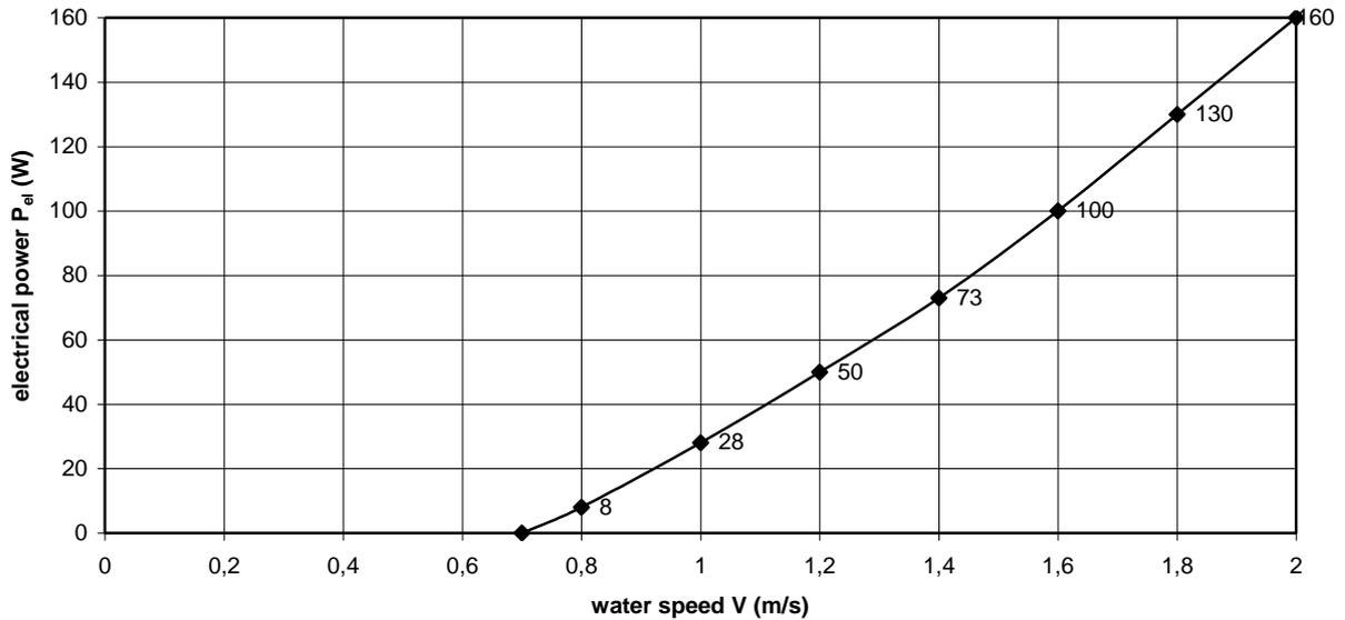
fig. 7  $P_{el}$ -V curve VIRYA-0.65 for 24 V battery charging
