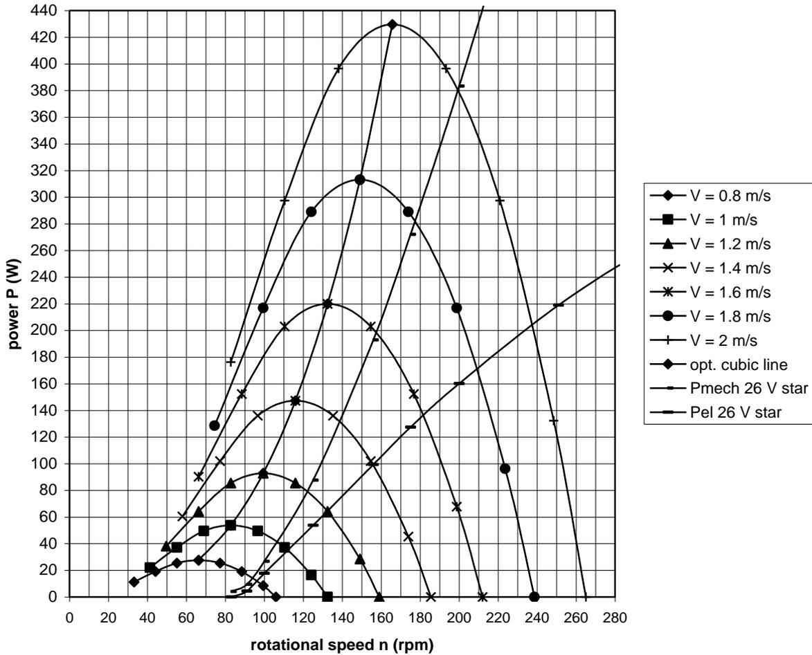
fig. 6 Calculated  $P$ - $n$  curves of the VIRYA-0.65 rotor for  $\delta = 20^\circ$  and measured  $P_{\text{mech}}-n$  and  $P_{\text{el}}-n$  curves of the generator for 26 V star
