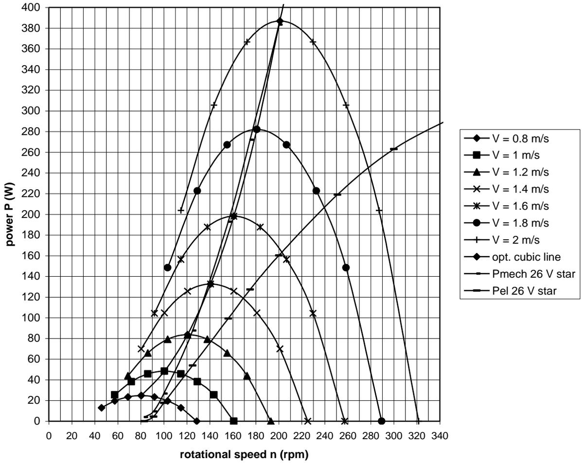
fig. 10 P-n curves of the VIRYA-0.625 rotor and optimum cubic line
