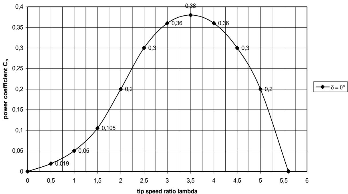
fig. 8 Estimated  $C_p$ - $\lambda$  curve for the VIRYA-0.625 rotor for the water direction perpendicular to the rotor ( $\delta = 0^\circ$ )
