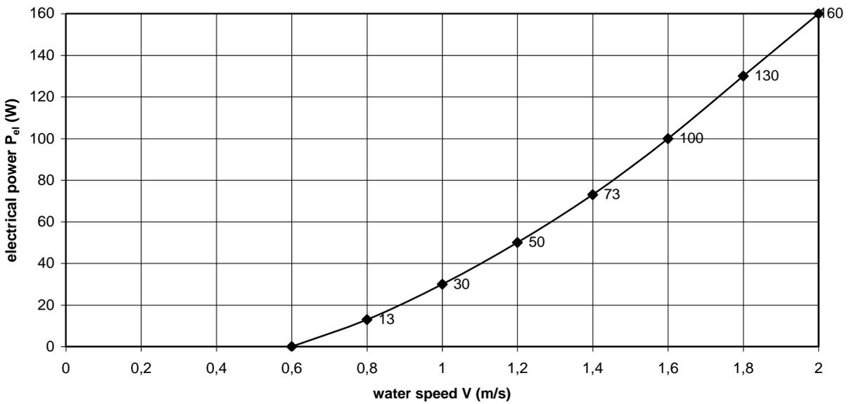
fig. 11  $P_{el}$ - $V$  curve VIRYA-0.625 for 24 V battery charging
