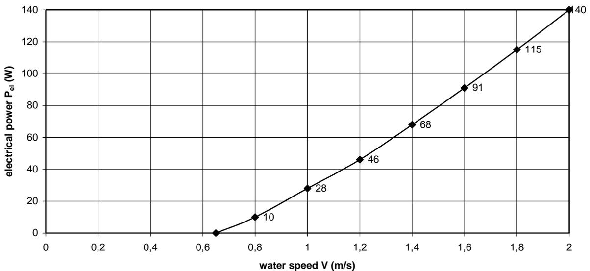
fig. 5  $P_{el}$ -V curve VIRYA-0.65 for 12 V battery charging
