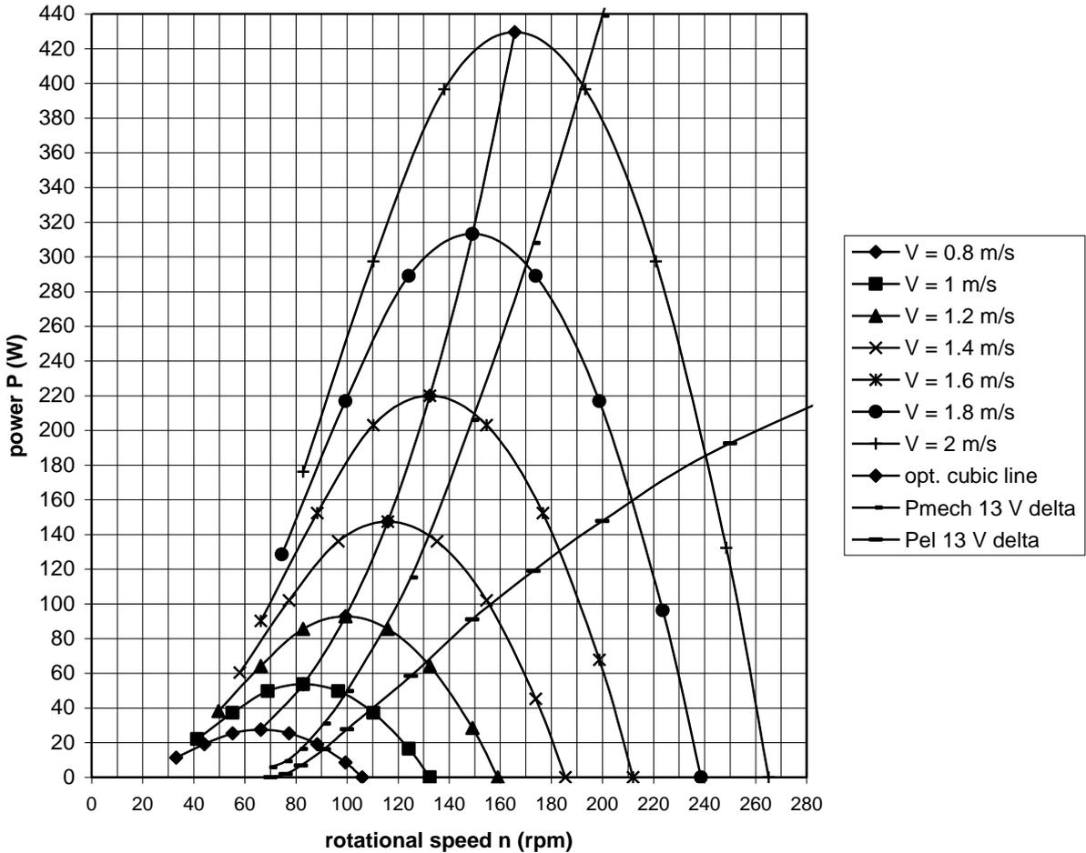
fig. 4 Calculated P-n curves of the VIRYA-0.65 rotor for  $\delta = 20^\circ$  and measured  $P_{\text{mech-n}}$  and  $P_{\text{el-n}}$  curves of the generator for 13 V delta
