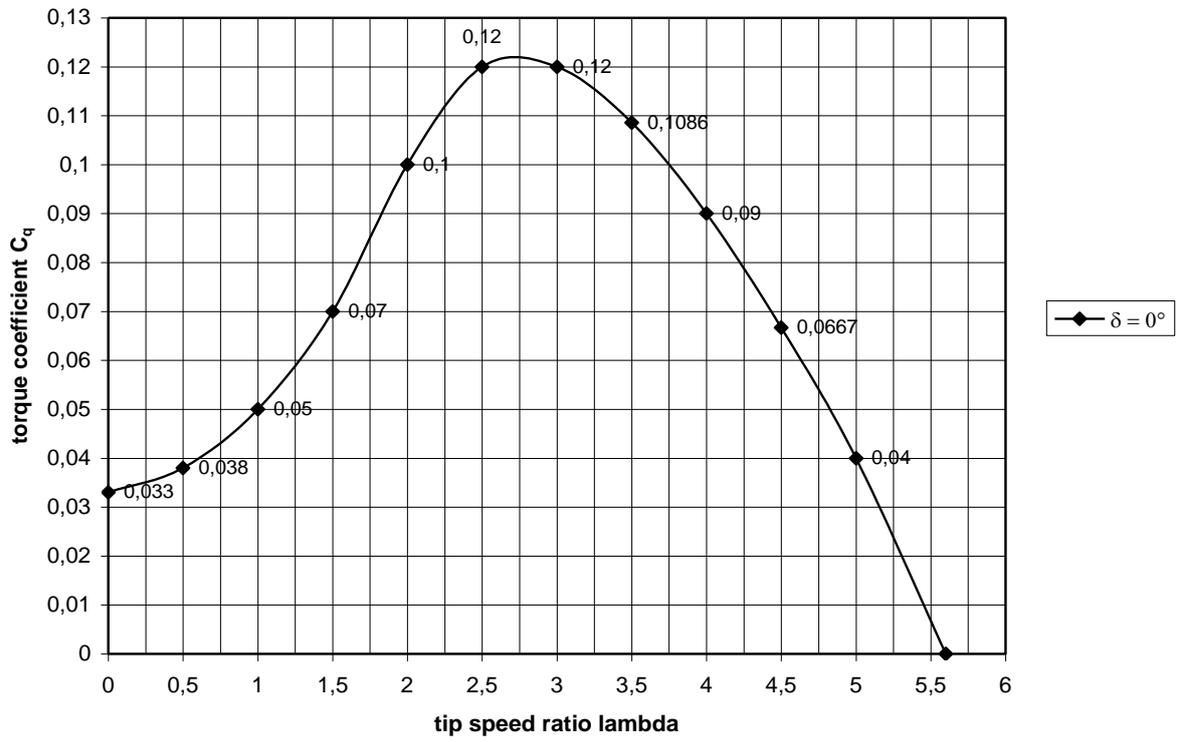
fig. 9 Estimated  $C_q$ - $\lambda$  curve for the VIRYA-0.625 rotor for the water direction perpendicular to the rotor ( $\delta = 0^\circ$ )
