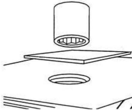
*A wrench socket drives the wet leather into the hole in the board.*
