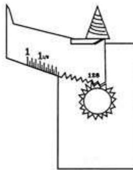
*An adjustable drill bit makes it easy to drill a hole just the right size.*
