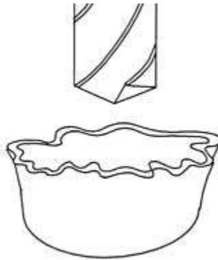
*Drill the hole for the seal retention screw.*
