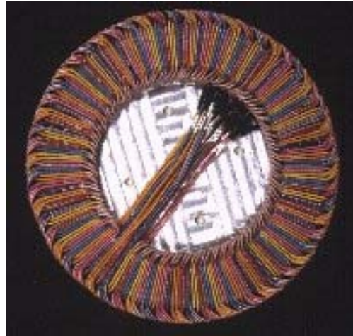
Stator winding
