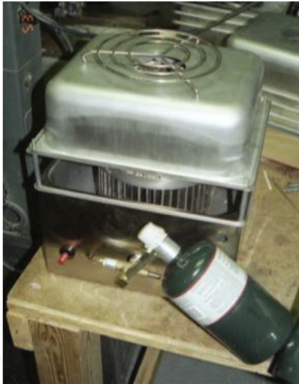
Figure 5. Schroeder-pulsed TE generator.
