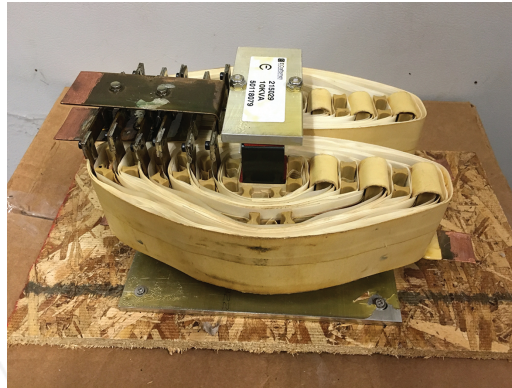
Figure 17. PWM 10-kW transformer dimensions 250 × 190 × 140-mm high.
