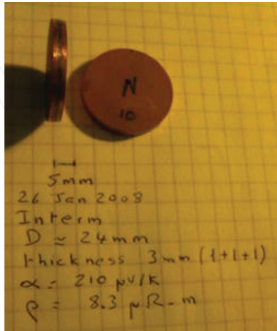
Figure 16. Bismuth telluride disc with copper caps.
